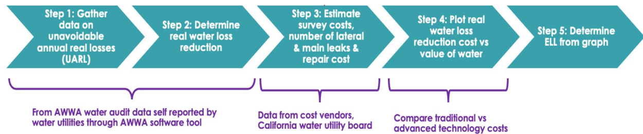
Figure 4. Cost assessment methodology to mitigate water main leaks and service connections.
