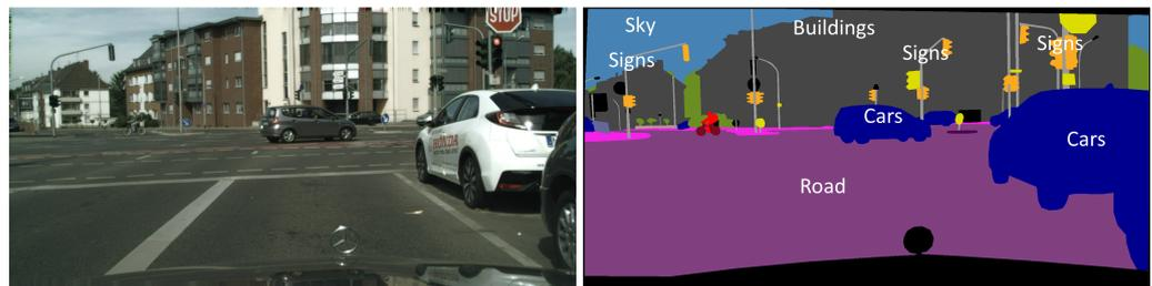
**Figure 1.** The Cityscapes dataset for autonomous driving semantic segmentation. Distinct regions are delineated by varying colors, each signifying unique object semantic information.
