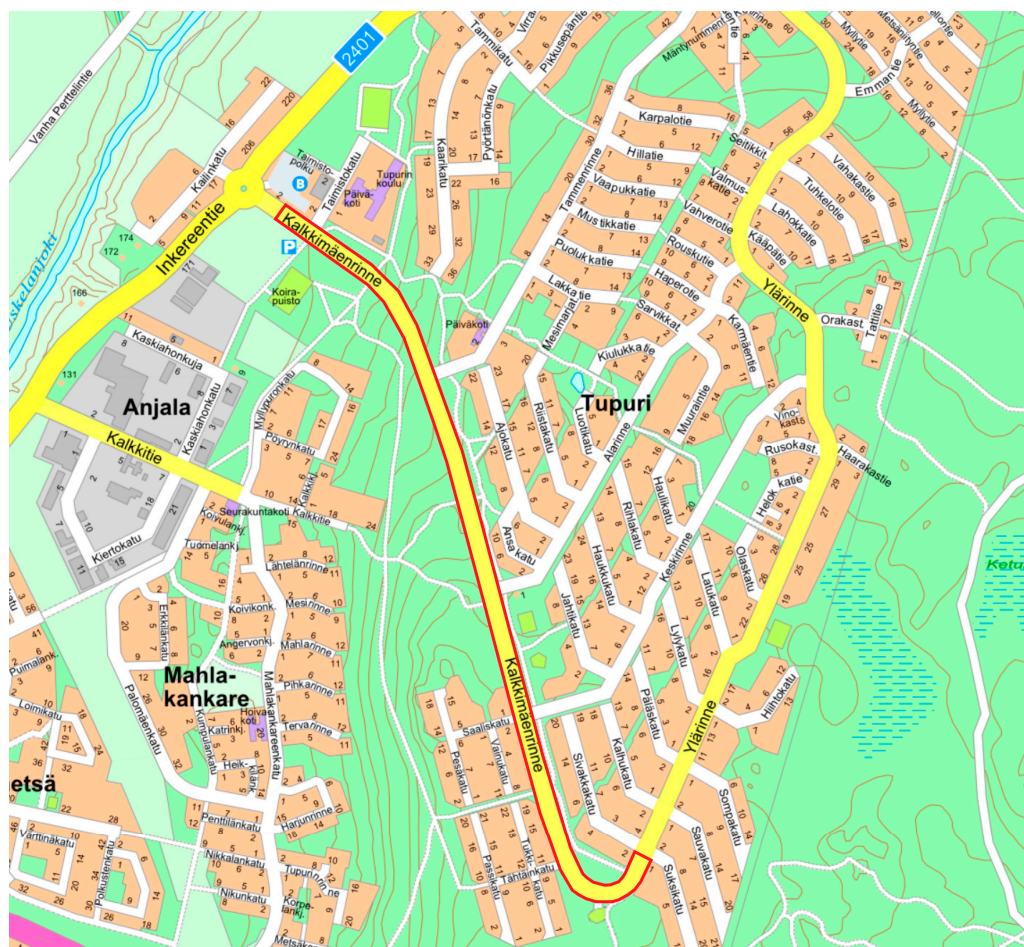
Figure 2. The map shows the collector road (Kalkkimäenrinne) test area in the context of the Tupuri housing area. The collector road had two-way traffic with one lane in each direction. The test area included one intersection, four T-junctions and six pedestrian crossings.
