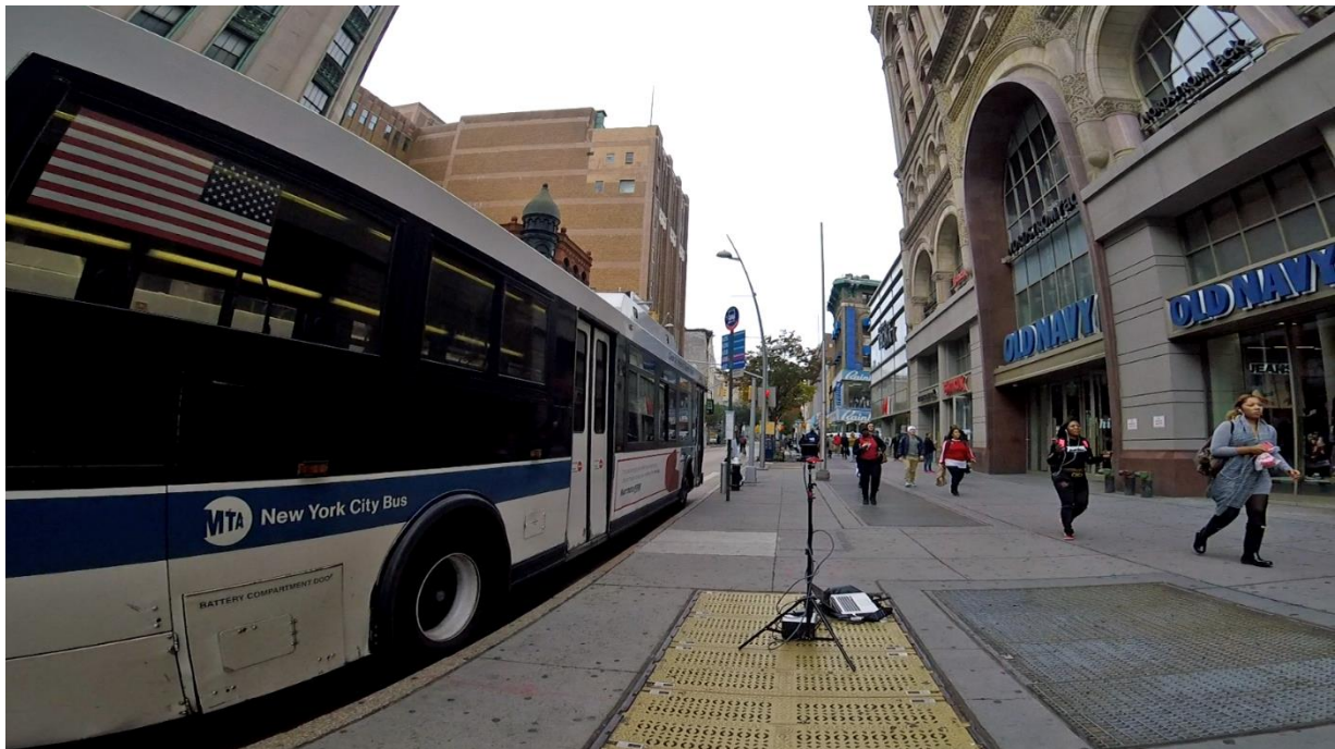
Figure 4. Automated analysis of pedestrian footfall on a retail high street with a LiDAR sensor positioned in the midst of high street dynamics.
