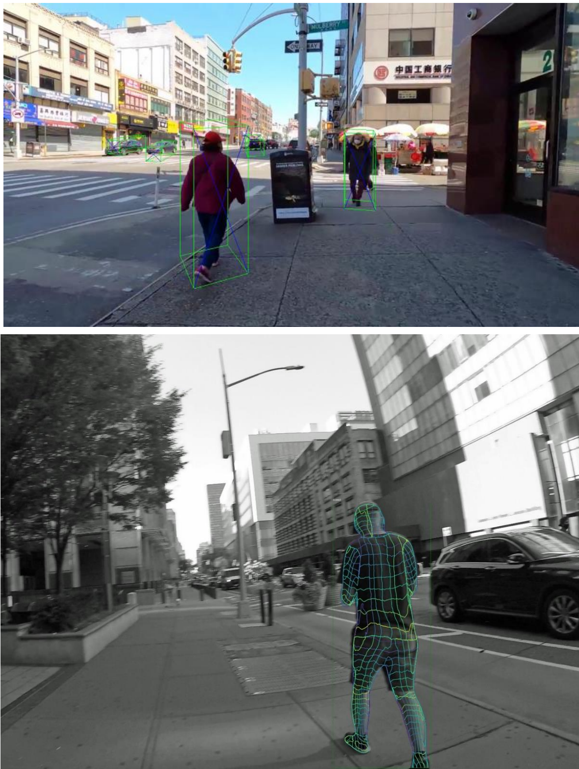
Figure 13. Pseudo-three-dimensional bounding ( top ) and mesh creation ( bottom ) of pedestrians and vehicles in a streetscape scene.
