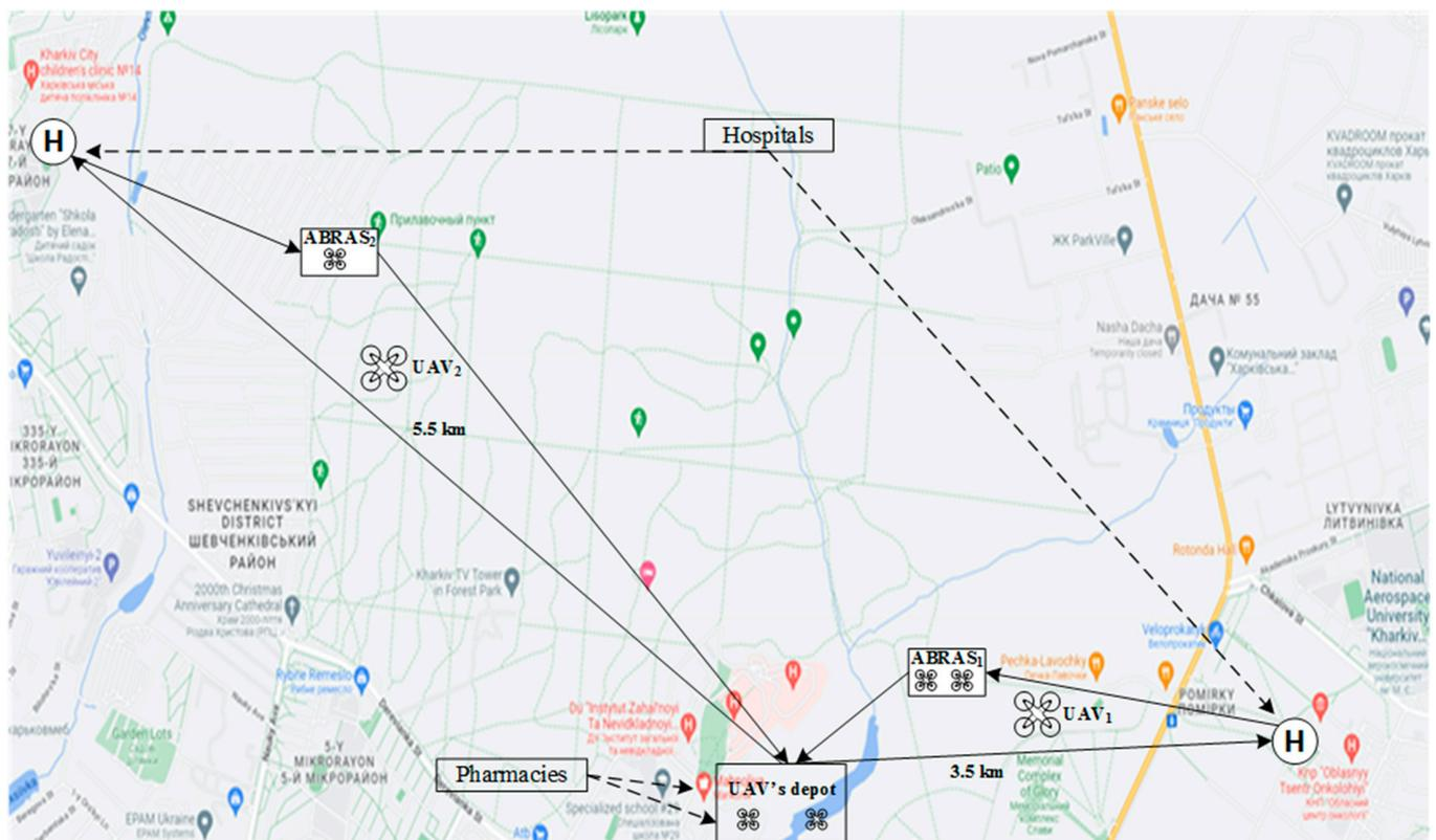
Figure 16. The scheme of UAVFaaS application for the delivery of medicines in the emergency mode.
