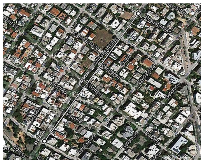
Figure 15. Antenna gain: 9 dBi; height: 5 m; BLE range: \approx 378 m.
