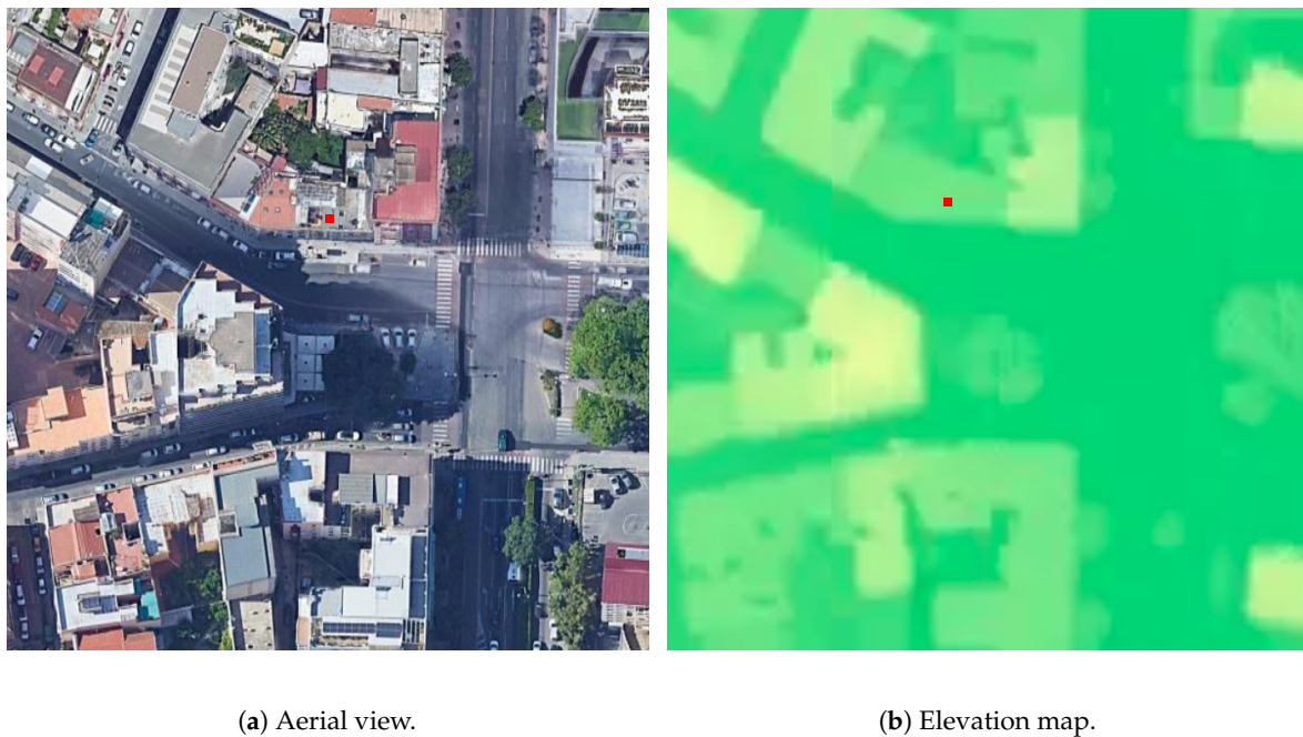
Figure 3. Satellite view and elevation map of the building chosen as an example and the surrounding area. The roof of the considered building (identified by the red point) is at a lower elevation than the buildings on its left and right, and also with respect to the building located on the other side of the street in the south-west direction.
