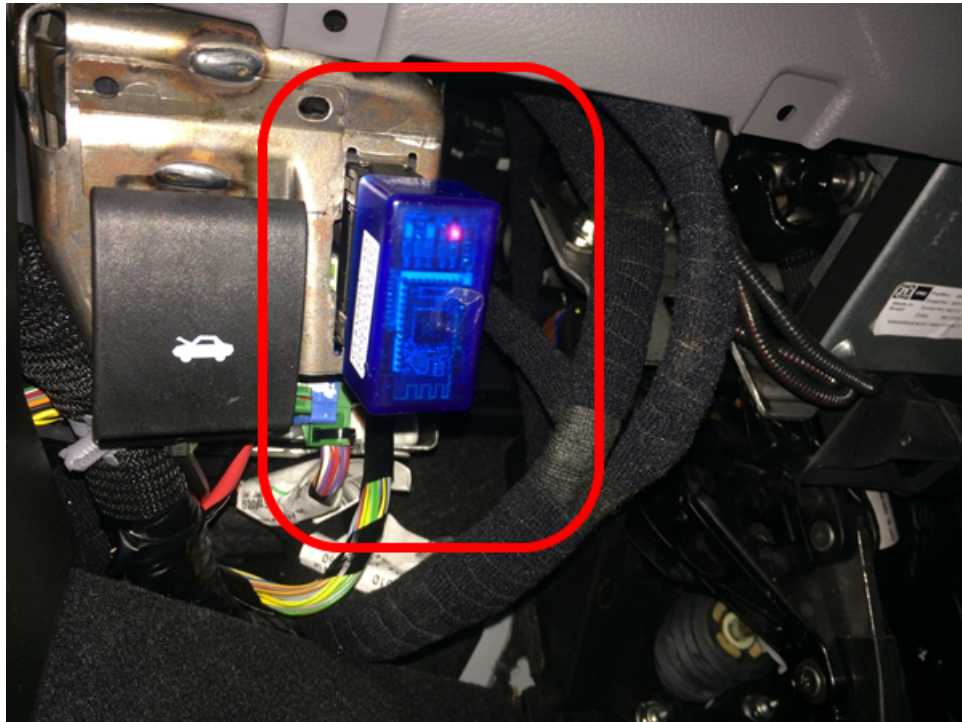
Figure 4. ELM327 connected to a OBD-II interface.
