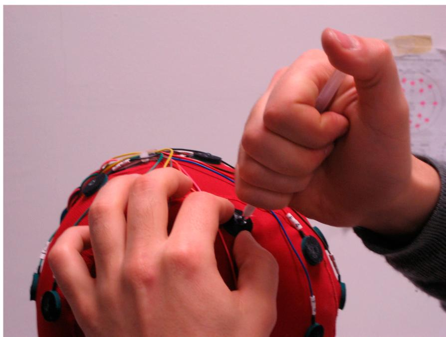
**Figure 1.** Detail of the experimental cap. Notice the introduction of the conductive gel into the electrode in the neoprene jacket.
