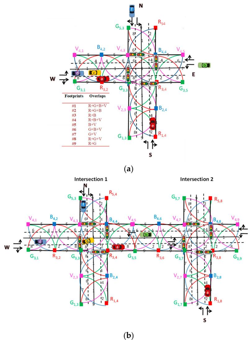
**Figure 2.** V2X optical infrastructure and generated joint footprints in a crossroad (LED array = RGBV color spots). (a) Standard intersection. (b) Split intersection.
