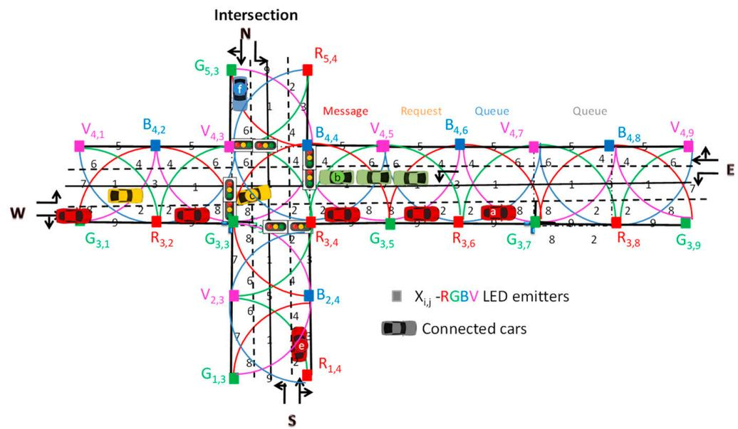
**Figure 10.** Simulated scenario: Four-legged intersection and environment with the optical infrastructure ( $X_{ij}$ ), the generated footprints (1–9) and the CV.
