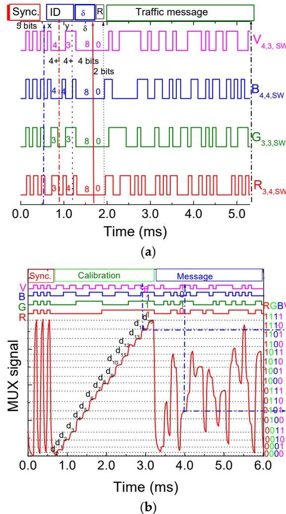
**Figure 6.** (a) Frame structure representation of a request message. (b) MUX/DEMUX signal of the calibrated cell. In the same frame of time, a random signal is superimposed.
