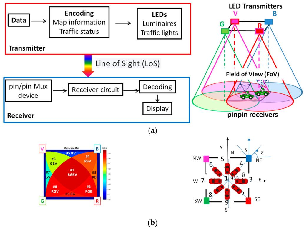
**Figure 1.** (a) Block diagram and transmitters and receivers and 3D relative positions of the VLC system. (b) Illustration of the coverage map in the unit cell: footprint regions (#1–#9) and steering angle codes (2–9).
