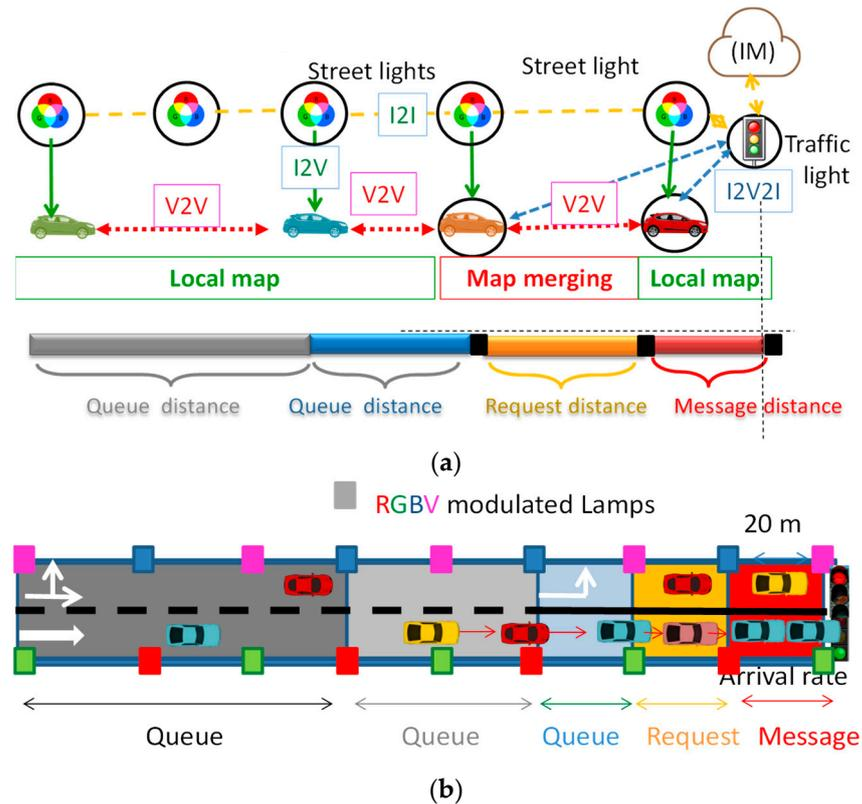
**Figure 4.** (a) Graphical representation of the simultaneous localization as a function of node density, mobility and transmission range. (b) Design of the state representation in the west arm of the intersection, with cells length.
