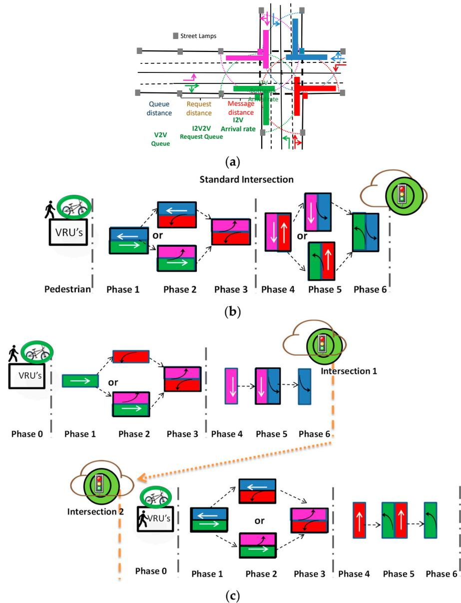
Figure 5. Phasing diagram: (a) Color poses. (b) Four-legged intersection. (c) Split intersection.
