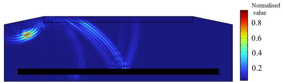
Figure 6. Cloud diagram of sound pressure in the air.
