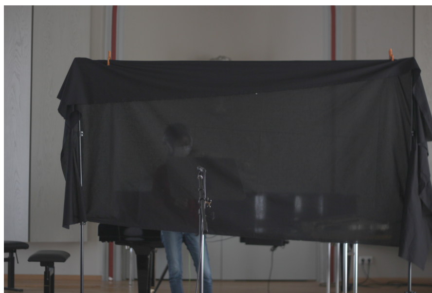
Figure 8. The setup for the live listening test with the musician situated behind an acoustically transparent curtain and wearing headphones playing white noise.
