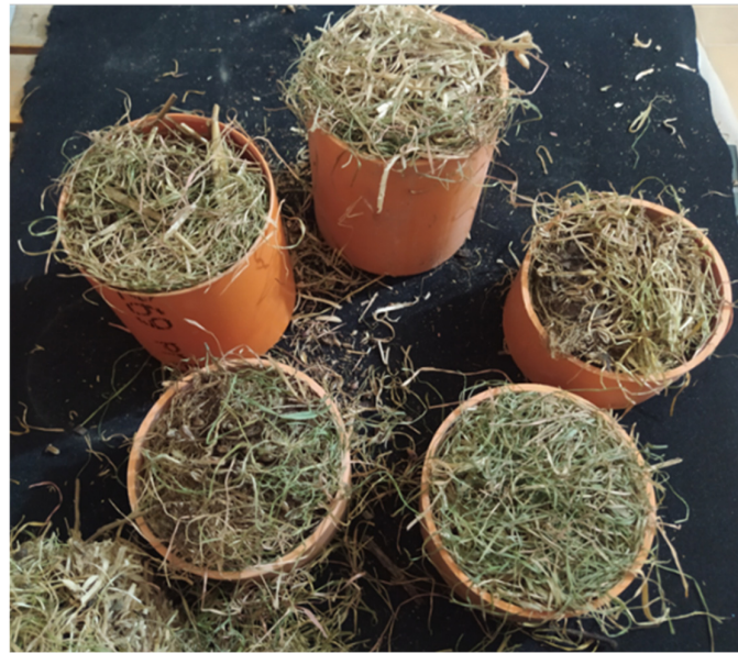
Figure 7. Hydroponic material samples ready for impedance tube measurements (5 cm and 10 cm thicknesses).
