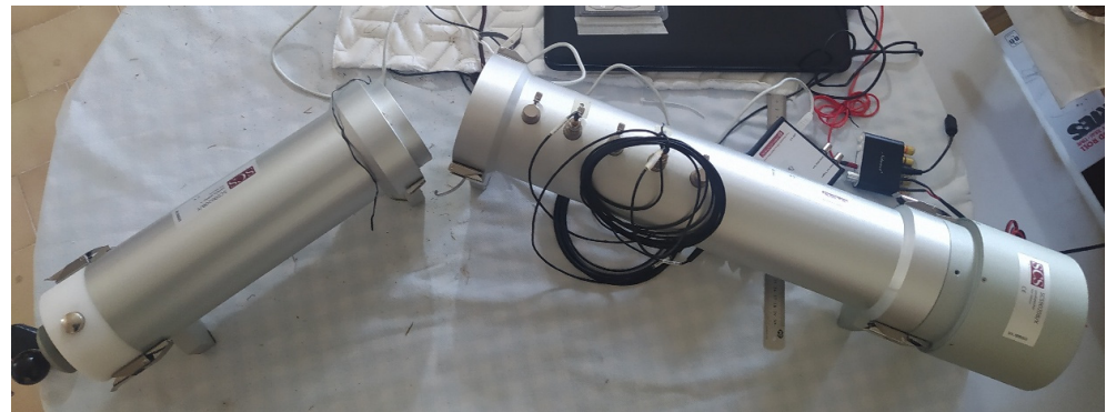
Figure 5. Impedance tube by SCS—SCS 902A.
