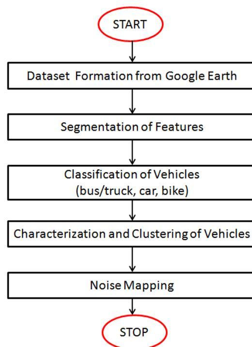
**Figure 5.** Flow diagram for automated noise dB calculation methods.
