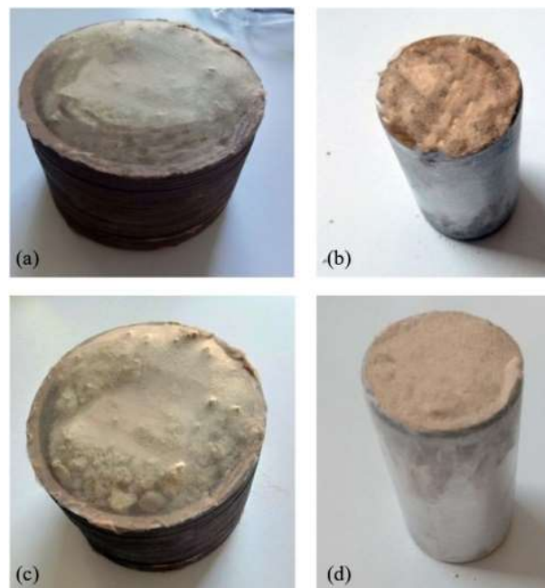
Figure 5. Göreme rock sample (a) for low-frequency setup; (b) for high-frequency setup; Ürgüp rock sample (c) for low-frequency setup; (d) for high-frequency setup.
