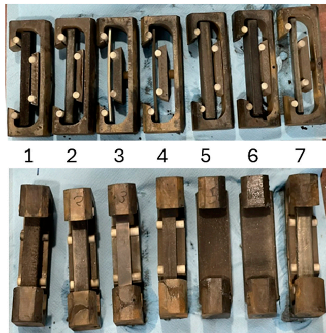
Figure 22. Samples in jigs 1 to 7 (according to Table 1). Samples #5 and #6 had no stress, samples #1 and #2 had a stress load level of 30% YS, and samples #3, #4, and #7 had a stress load level of 100% YS.
