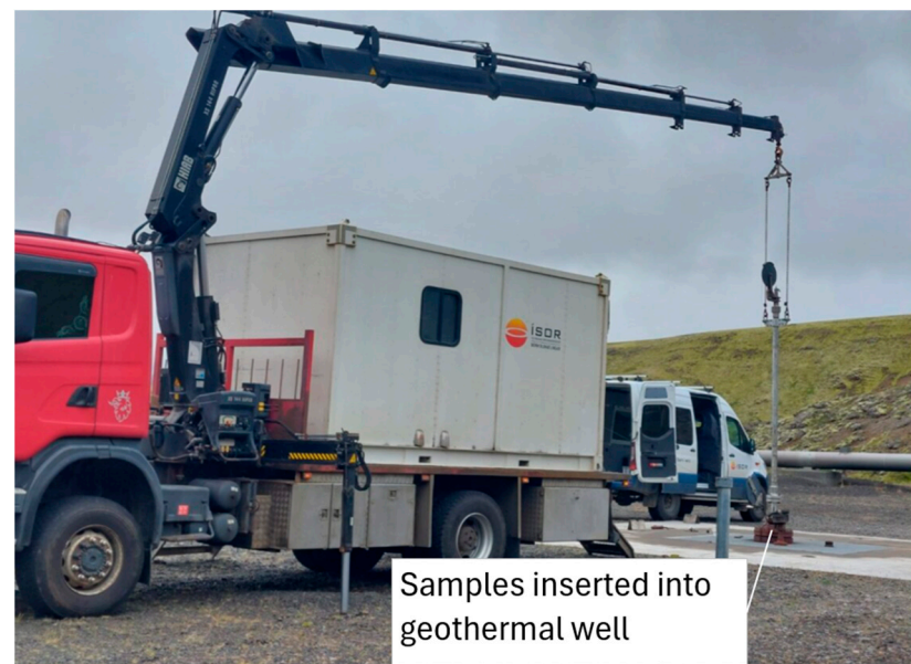
Figure 7. Samples in the sample holder unit were inserted down to a 1300 m depth in well HE-52, where the temperature was 262 °C and the pressure was 95 barG.
