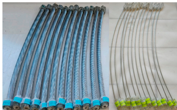
Figure 1. Test specimens (strands, wires) for corrosion.
