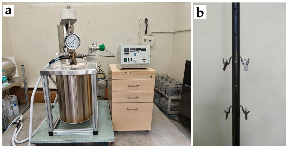
**Figure 4.** (a) steam oxidation experimental test facility; (b) sample holder with coupons.
