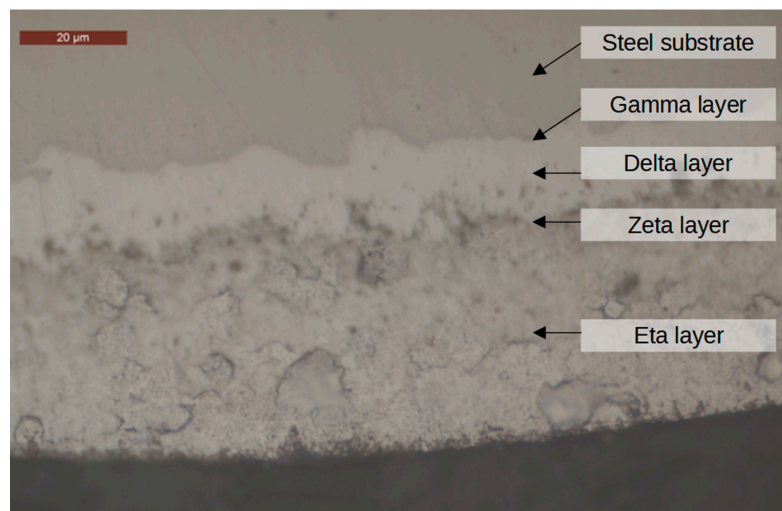
Figure 5. Intermetallic layers in the steel substrate.
