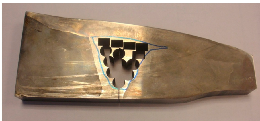
Figure 2. Dissimilar metal weld of Alloy 182 between SA-508 (left) and 316 L (right).
