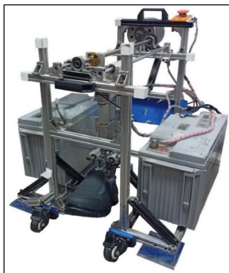
Figure 3. Whole-shoe portable slip tester.
