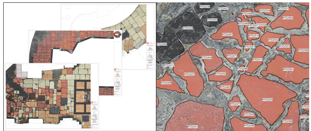
Figure 7. Operational use of the federated HBIM system during the conservation works. (Left): documentation sheets automatically generated from the FloorTilesModel to support on-site data collection. (Right): detail of a documentation sheet showing the unique BIM identifier (ID) assigned to each floor tile. The same identifier is used to associate conservation records collected during the intervention with the corresponding HBIM element, enabling the automatic reintegration of updated information into the federated model.
