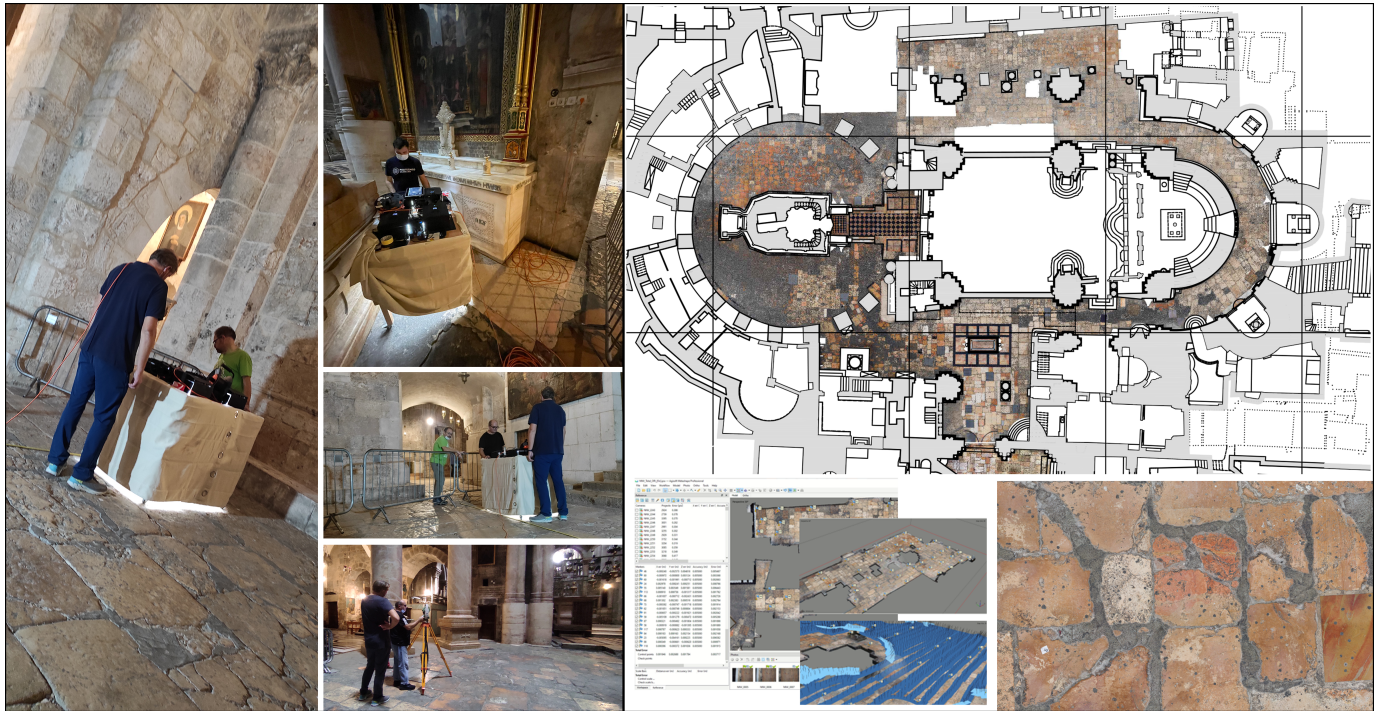
Figure 1. Photogrammetric survey workflow adopted for the documentation of the Basilica floor. (Left): field acquisition using the custom mobile photogrammetric prototype developed by Politecnico di Milano, showing representative surveying operations and examples of the conservation condition of the pavement. (Right): photogrammetric processing in Agisoft Metashape (the language of the software was set to Italian, so the text in the screenshot is Italian, but it is not meaningful for the content of the image), including image alignment, dense point cloud generation, and the resulting high-resolution orthophoto of the Basilica floor, with a detail of the final orthophoto.
