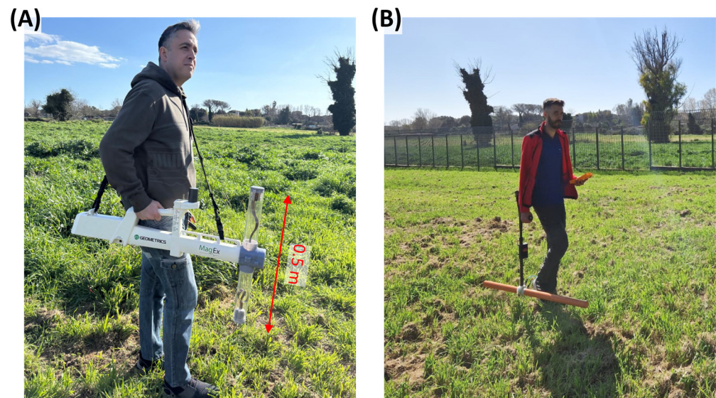
Figure 2. Geophysical equipment. (A) Geometrics Micro-Fabricated Atomic Magnetometer gradiometer prototype and (B) GF Instruments CMD-Mini Explorer electromagnetic conductivity meters. Red arrow indicates the distances between the magnetic sensors.
