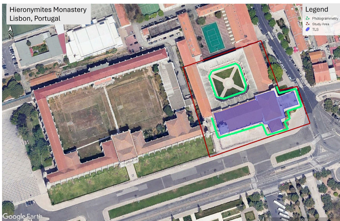
Figure 1. The Hieronymites Monastery in Lisbon [44]. The red line shows the study area; the green line shows the areas surveyed by photogrammetry; and the blue polygon shows the areas surveyed by Terrestrial Laser Scanning.
