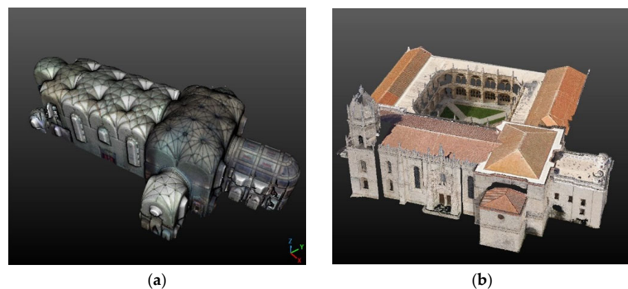
Figure 3. Point-clouds of the Hieronymites Monastery: (a) TLS surveyed interior, (b) Photogrammetric surveyed exterior; roofs obtained from virtual flight.
