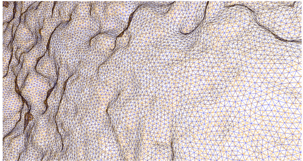
Figure 6. Before (orange) and after (blue) remeshing, with mesh wireframes superimposed.
