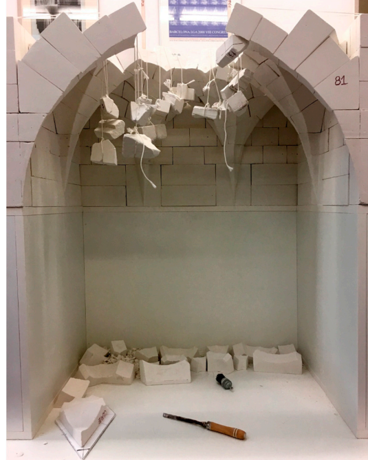
Figure 6. Navarro's hypothesis on how to complete the vault. Source: Author's own work.
