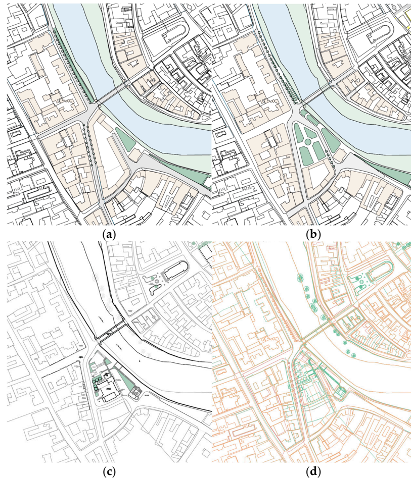
Figure 7. (a) Town's plan from 1934; (b) town's plan from 1950; (c) town's plan from 2023; (d) overlap of all three plans; all plans are reconstructed based on historical photographs and on-site measurements [27].
