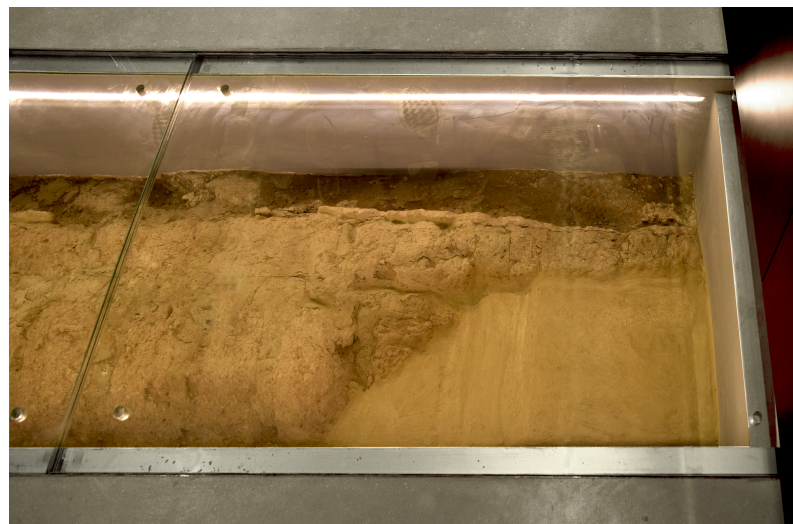
Figure 3. Detail of an earthen remain. The uneven shape makes it difficult to assess deterioration by visual inspection.
