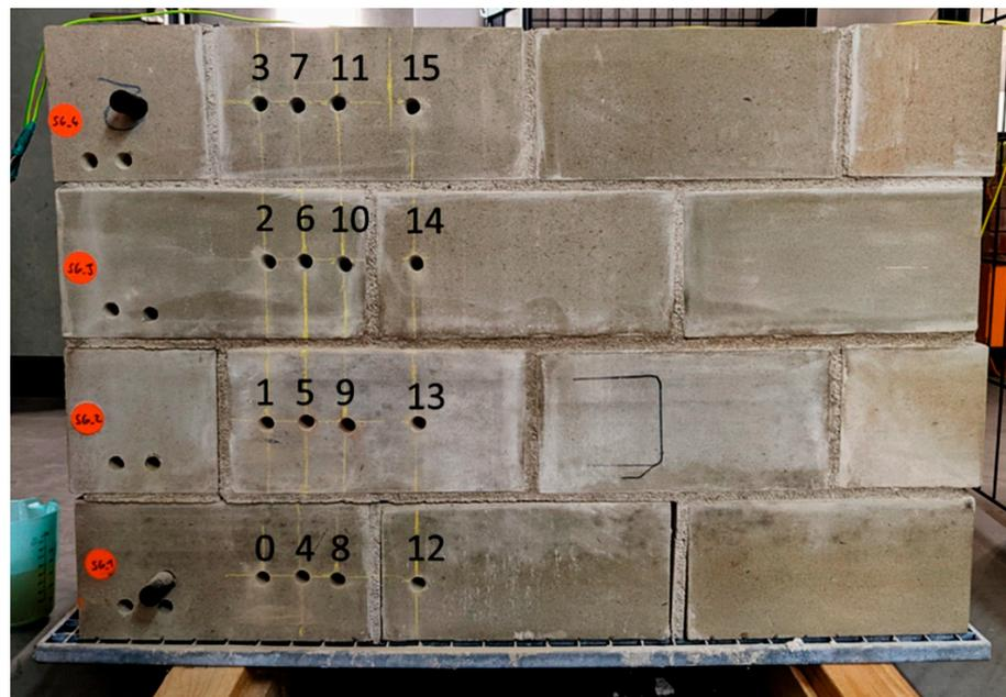
**Figure 13.** Equidistant extraction points of the four measurement days resulting in a total of 16 individual positions.
