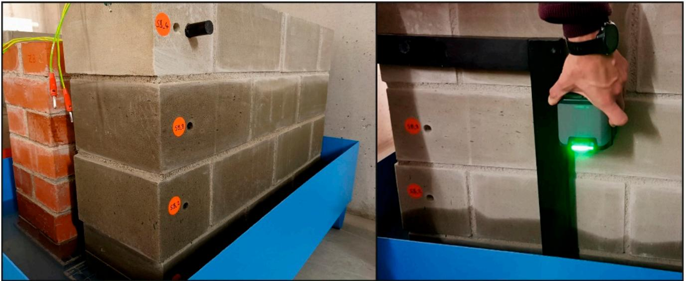
**Figure 7.** (Left) Masonry shortly before the water was drained. The suction horizon on the sandstone masonry can be seen very clearly. (Right) Radar measurement along the positioning frame.
