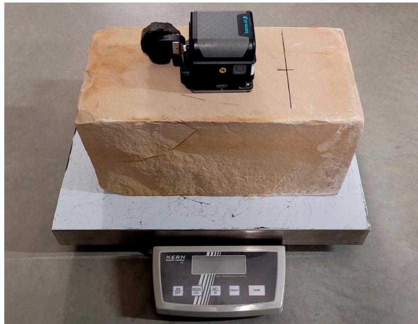
**Figure 5.** Measurement of the drying process of individual bricks along an axis with the radar device. Continuous weight measurement allows conclusions to be drawn about the water content in the sample.
