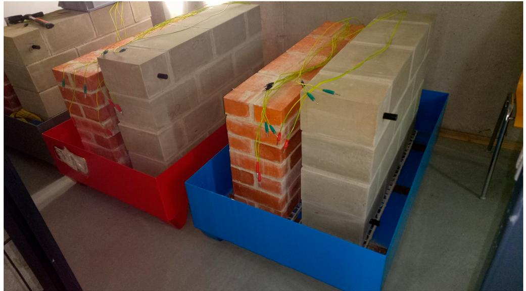
**Figure 3.** Stored test specimens in steel profile troughs.
