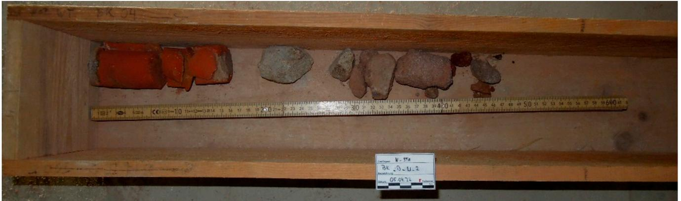
**Figure 17.** Drill core taken from a single-shell vault masonry of the state archive in Nuremberg. The sample number here is BK\_B\_W\_2.
