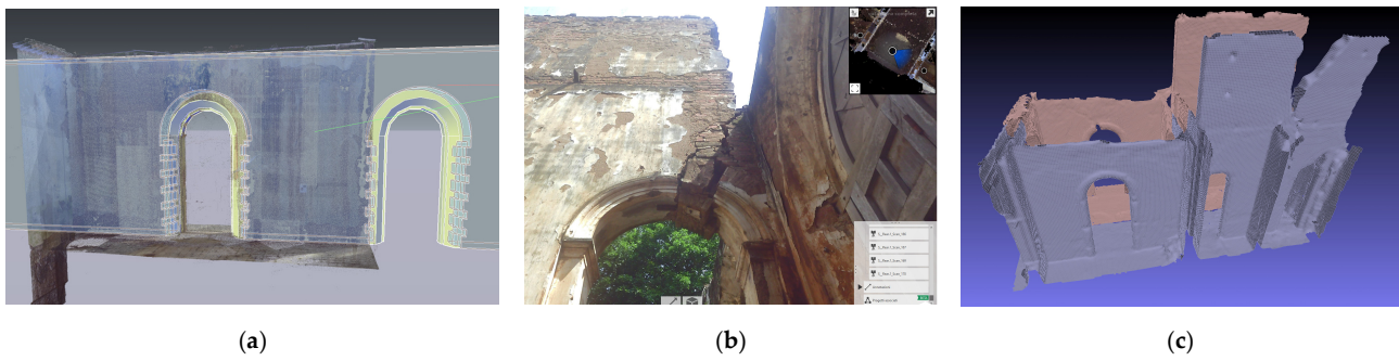
Figure 13. (a) Geometrical model of the wall simplified into geometry: from a triangulated mesh to a quadrangulated mesh with a window inserted; (b) real-view image in recap software of a damaged wall; and (c) a simplified model of the same damaged wall.
