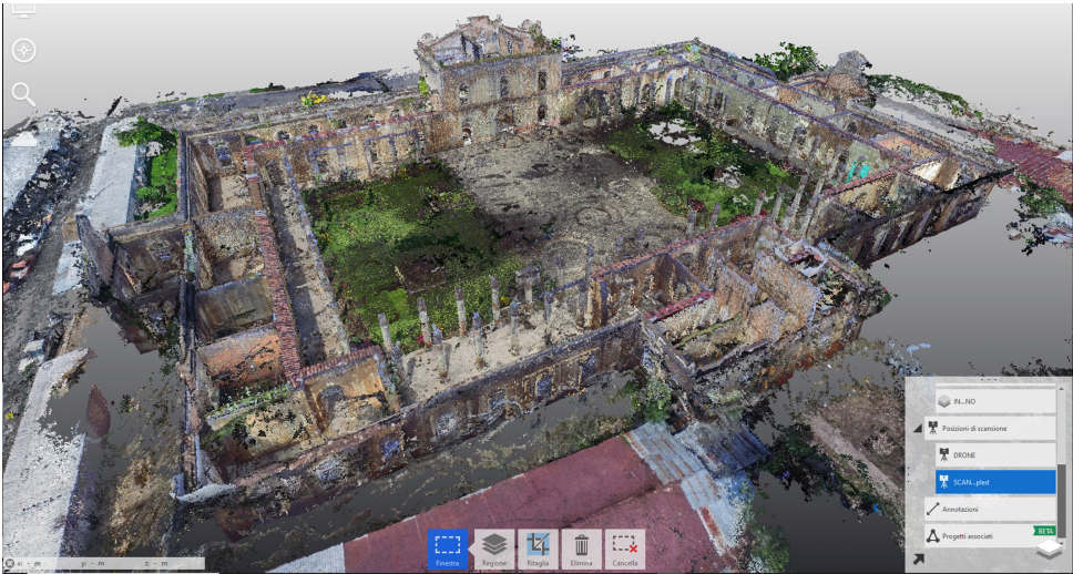
Figure 8. Overall view of the structured point cloud, considering the alignment of the laser scanner point cloud and the drone point cloud.
