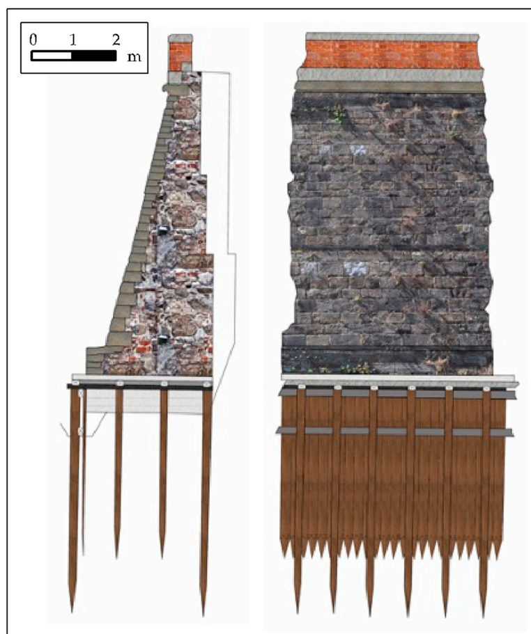
Figure 2. Construction techniques of the Lungarno Torrigiani riverbank (modified from original drawings preserved in the municipal historical archive of Florence).
