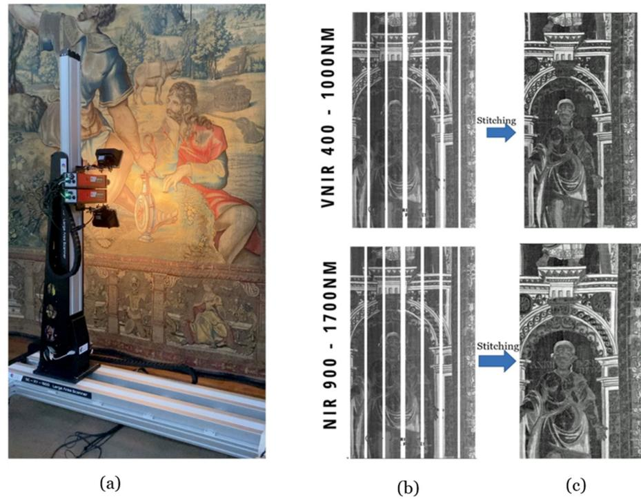
**Figure 3.** The hyperspectral imaging scanner set up in front of the *Sacrifice of Isaac* tapestry in the Great Hall, Hampton Court Palace, UK (a) The hyperspectral image strips from the VNIR and NIR cameras (b) The composite hyperspectral images in VNIR (top) and NIR (bottom) (c).
