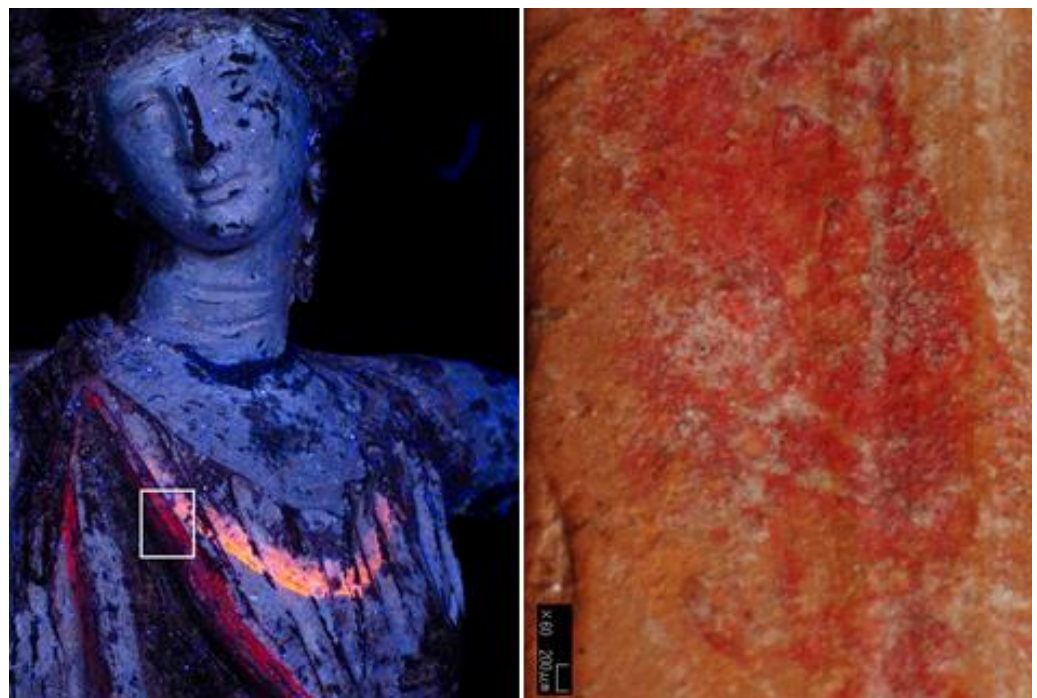
Figure 15. UIL image and microphotograph ( \times 60 ) of the vivid red paint on the overfold: madder atop (or mixed with) cinnabar © G. Verri (UIL) and C2RMF/B. Bourgeois(microphotograph).
