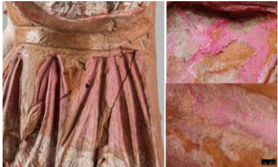
Figure 19. Pink madder on dress: directly on clay (upper right) or atop an orange-salmon underlayer (lower right). © C2RMF/B. Bourgeois (microphotographs ( \times 60 )).
