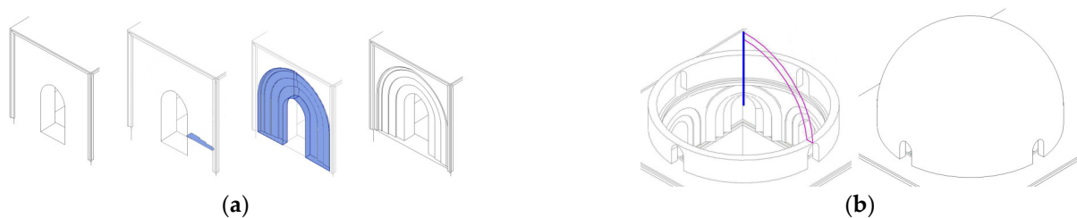
Figure 15. Features created by a combination of Revit tools: (a) sweep plus extrusion from a profile, (b) revolve from a profile.
