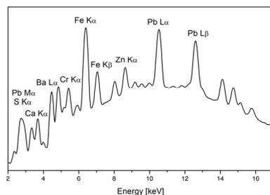
**Figure 1.** XRF spectra of *Green Cinnabar* paint (a mixture of Prussian blue with chrome yellow) from the tube.
