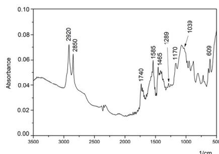
**Figure 2.** FTIR spectra of red organic dye (*lacca*) deposited on barium white from the tube.
