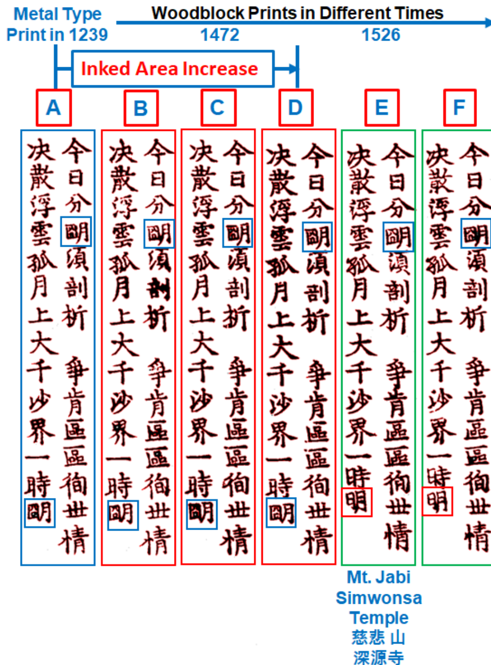
Figure 5. Printed characters were extracted and highlighted by red outlines using PicMan for character shape inspection and inked area measurement. Two characters of 明 highlighted by red squares on the bottom right have been changed from an old-style character 明 to a new-style character 明 during woodblock duplication by the engraver. (A) Gongjin version (空印本), (B) Banyasa Temple version (般若寺本), (C) Daegu version (大邱本) 1472, (D) Samseong version (三省本), (E) Jongno Public Library version (鍾路圖書館本) 1526 and (F) National Library of Korea version (國立中央圖書館本)).
