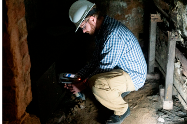
Figure 10. Taking PRXF readings on the lead lining of the coffins and on the coffin fittings in the St. Patrick's Church crypt vaults.
