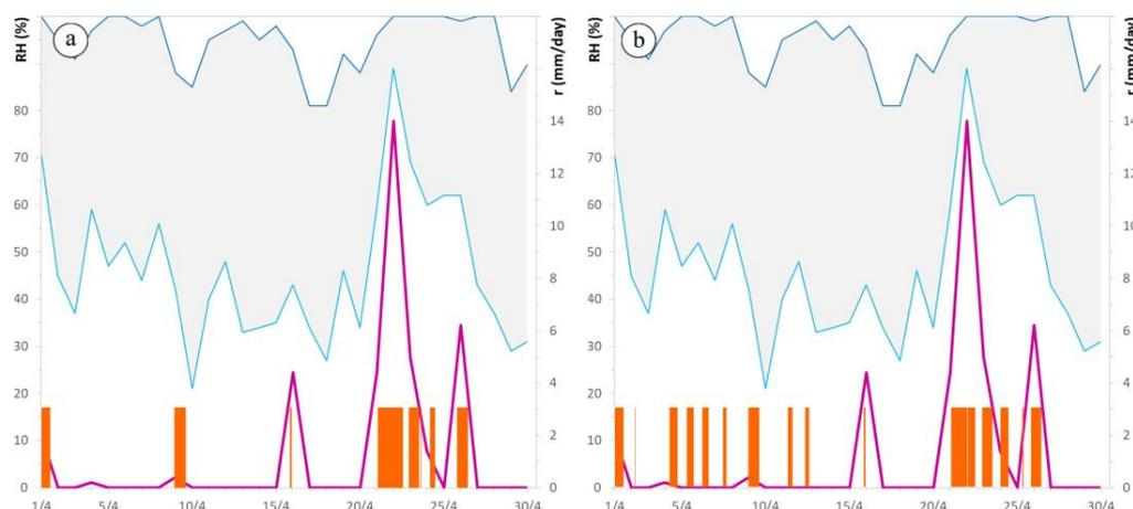
**Figure 6.** RH (gray area with maxima in dark blue and minima in light blue), daily precipitation  $r$  (purple), and surface moisture of a spruce sample (orange bars), with (a) unfinished and (b) finished surface, measured in the pilot site of Padova in April 2022. NB: the moisture data are dimensionless and binary; the bar indicates every time the material surface is wet.
