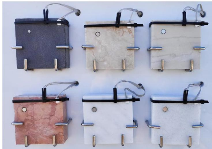
**Figure 2.** The surface sensors mounted on the samples.
