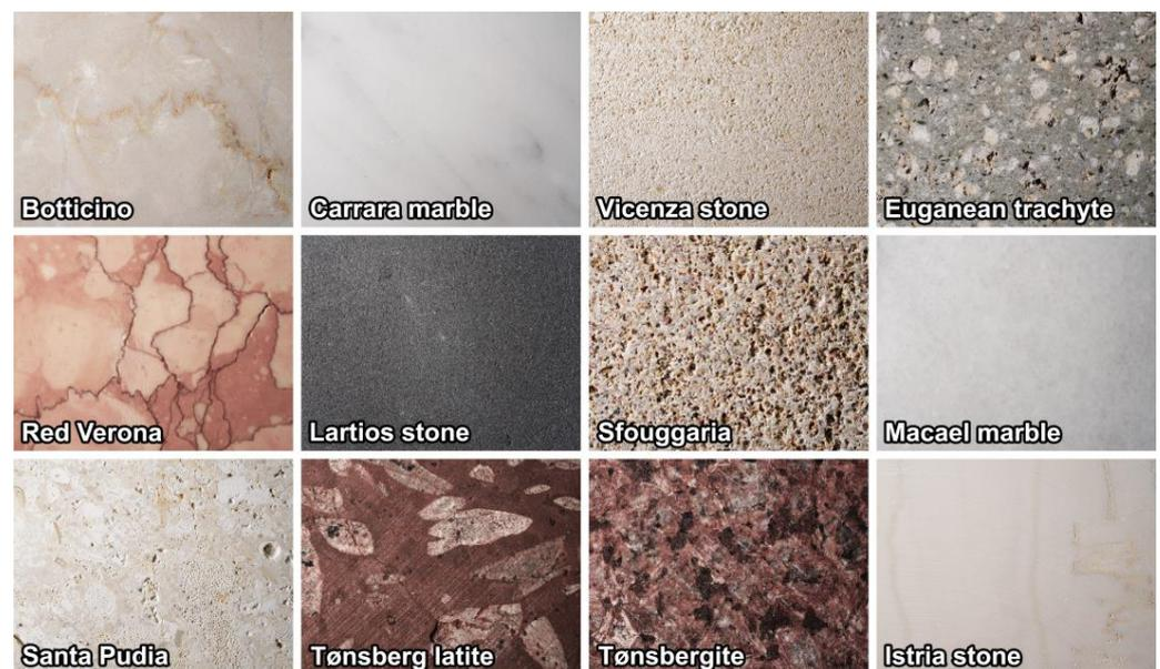
**Figure 1.** The stone materials selected (the short side of each photo is 4 cm).
