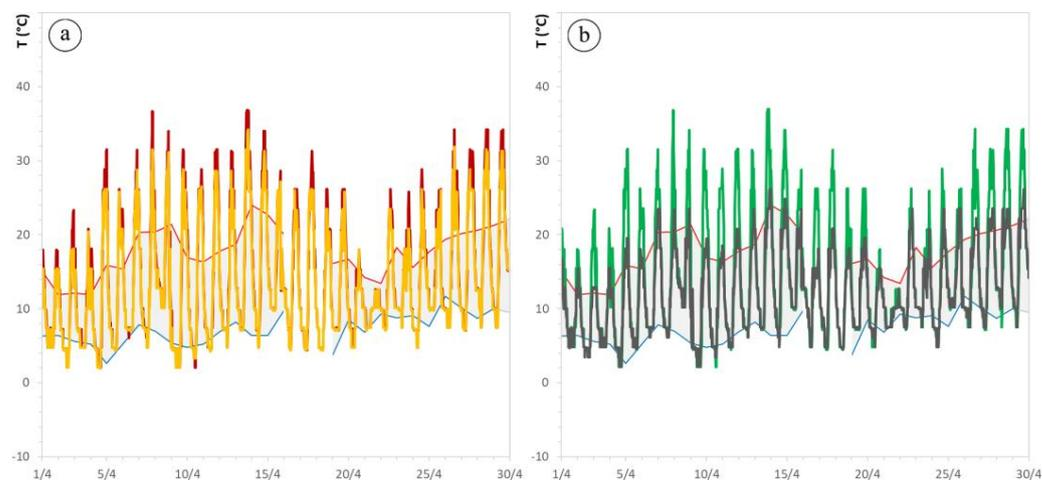
**Figure 5.** Air temperature (gray range with maxima in light red and minima in blue) vs. stone surface temperature, measured in the pilot site of Padova in April 2022; (a) trends of two different materials (dark red: Lartios stone; orange: Macael marble); (b) the same material (Lartios stone) at different orientations (dark gray: N exposure; green: S exposure).
