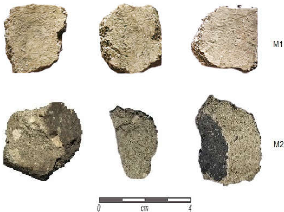
Figure 2. Samples from Corvins' Castle—DT: (M1 and M2) masonry mortars. M1 is collected from the inside of the tower, while M2 is collected from outside of the castle.
