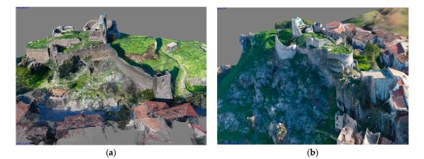
Figure 11. (a) Dense cloud model: View from the east. (b) 3D textured mesh model: View from the south-west.
