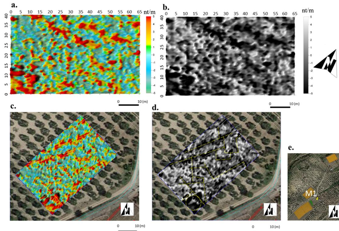
**Figure 6.** MAG maps acquired in correspondence to the area M1 (e), in false color (a), and in grey scale (b), superimposed on a satellite image (Google Earth 2018) (c,d) with the most interesting alignments indicated with yellow lines.
