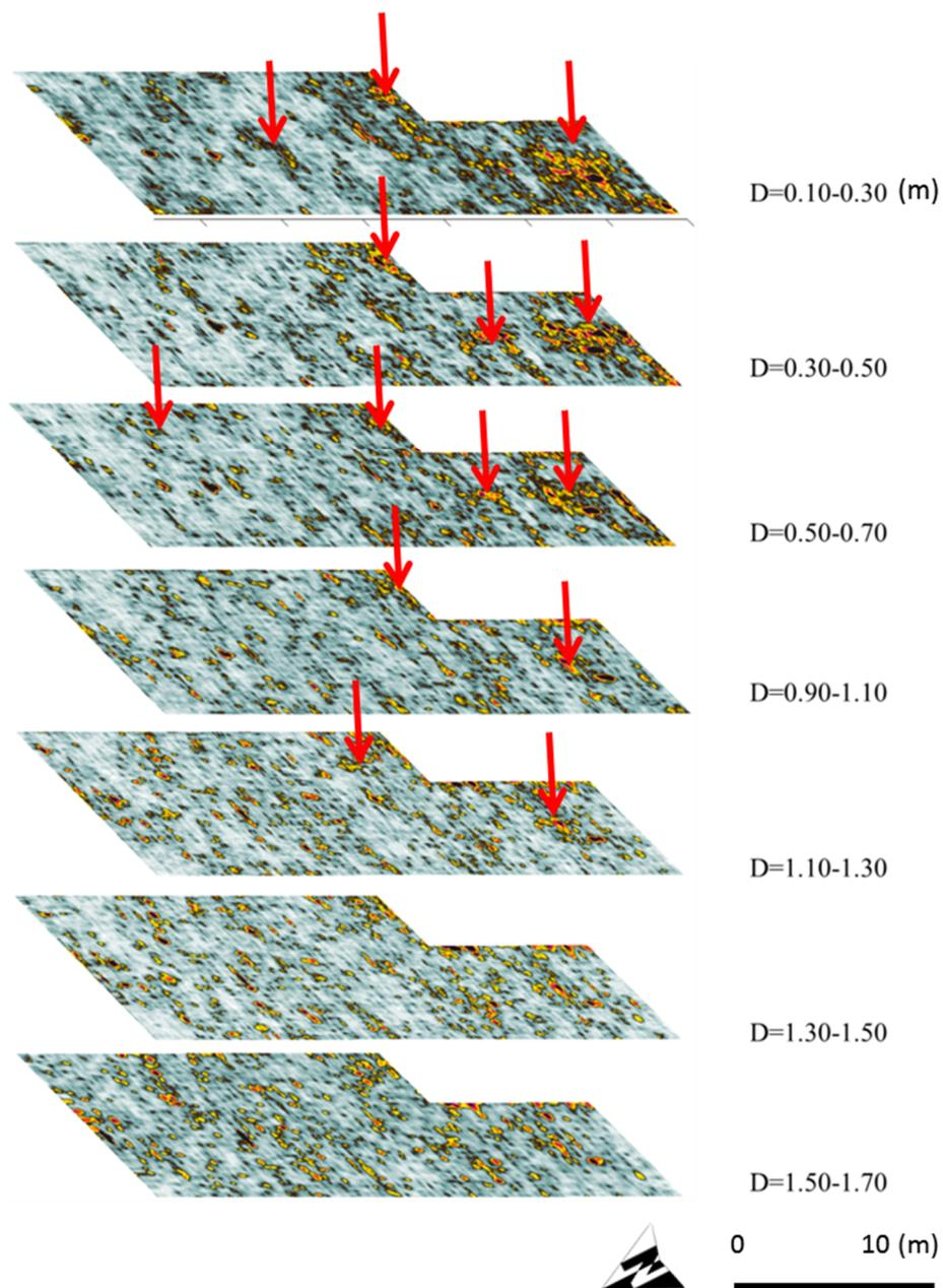
**Figure 9.** GPR depth slices extracted from the 3D model of area G1, with red arrows indicating the more interesting reflections in the first meter investigated.
