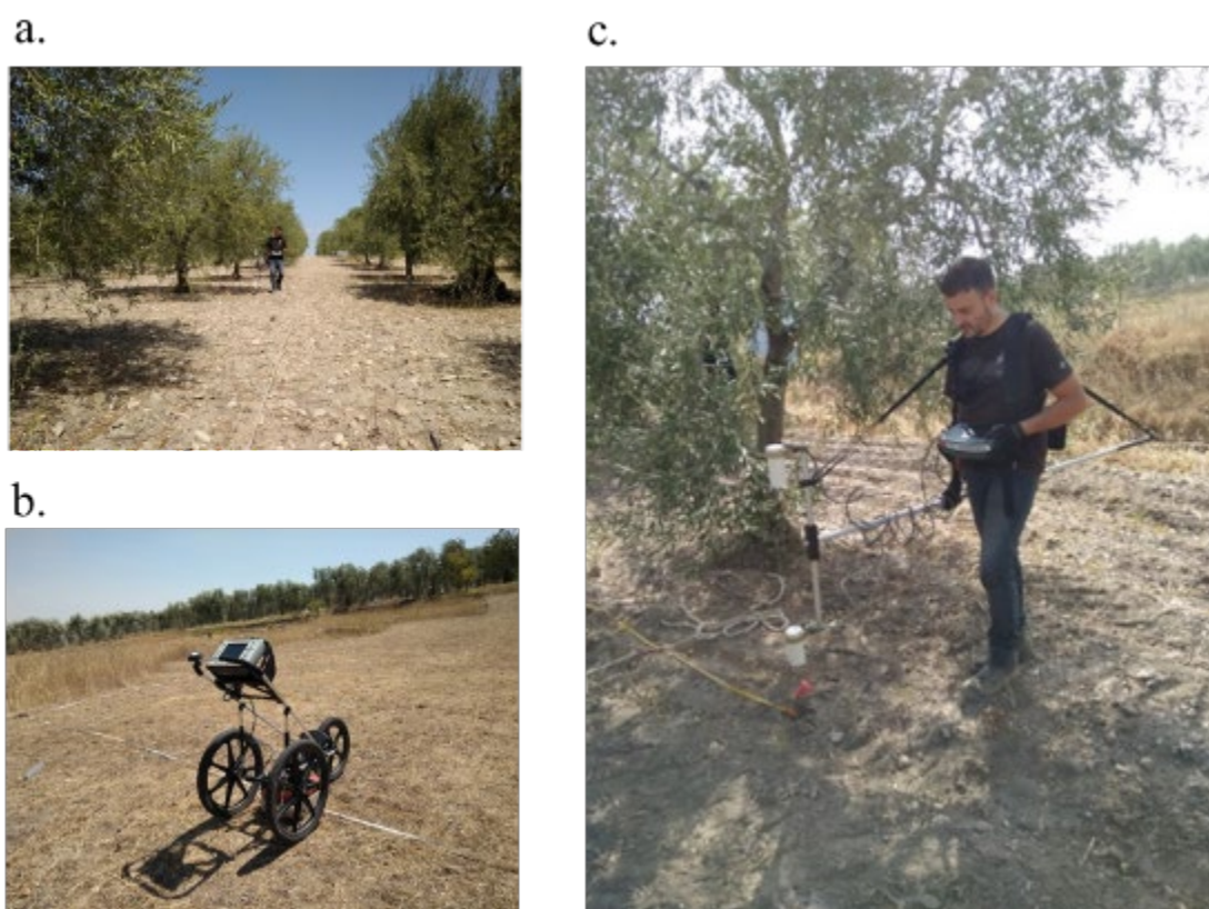
Figure 5. Geophysical readings at the site of Forentum ; most of the area investigated is characterized by its olive groves (a) and was investigated using a ground penetrating radar (GPR) mounted on a cart (b), while in (c), the cesium vapor magnetometer used for the gradiometric configurations (MAG) readings is analyzing position M3 on the map.
