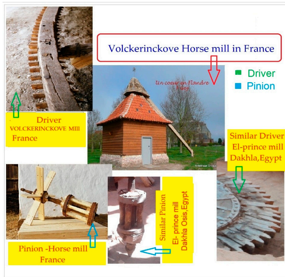
Figure 9. Comparison between the Horse-drawn mill of Volckerinckove in France and other animal powered mills in our Oasis. There are some copies in Belgium. Association Yser Houck rebuilt it in 2009–2010.
