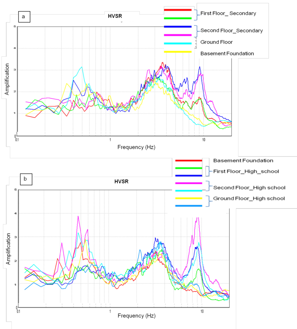
Figure 9. HVSR estimated at each floor of the secondary school (a) and the high school (b).
