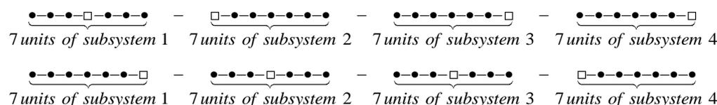
**Figure 3.** Failure scenarios for the series network  $NET(4,2,3,7)$ .
