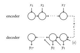
Figure 3. Encoder-decoder sequence to sequence model.
