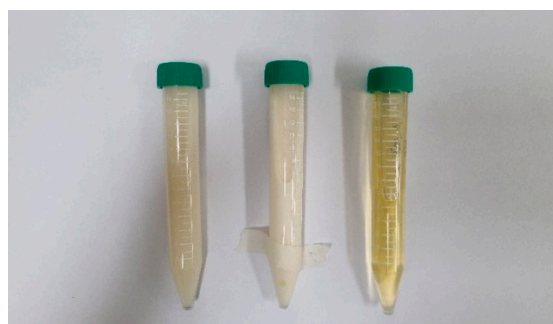
Figure 17. Visual appearance of SCFs under different initial pH conditions: pH 7 (left), pH 4 (middle), and pH 2 (right).
