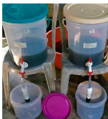
Figure A2. Filter columns with adsorbent SSW and commercial activated carbon.
