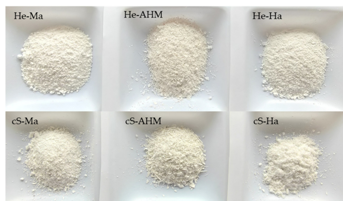
Figure 1. Mineral fraction obtained after hydrolysis and calcination of heads (He) and central skeletons (cS) of mackerel (Ma), Atlantic horse mackerel (AHM), and Hake (Ha).
