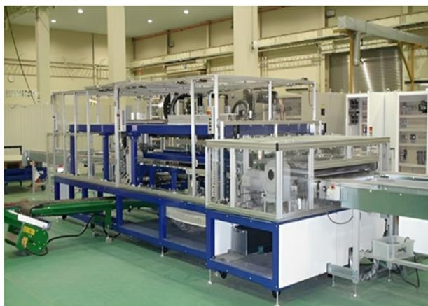
**Figure 6.** Module delamination involves glass and EVA separating equipment (Photo courtesy of NPC Incorporated) [20].
